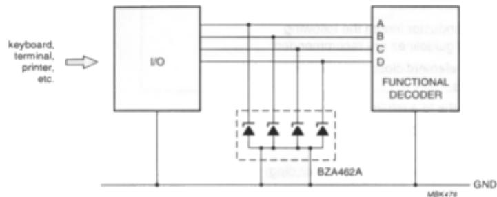
Fig.7 Computer interface protection.
