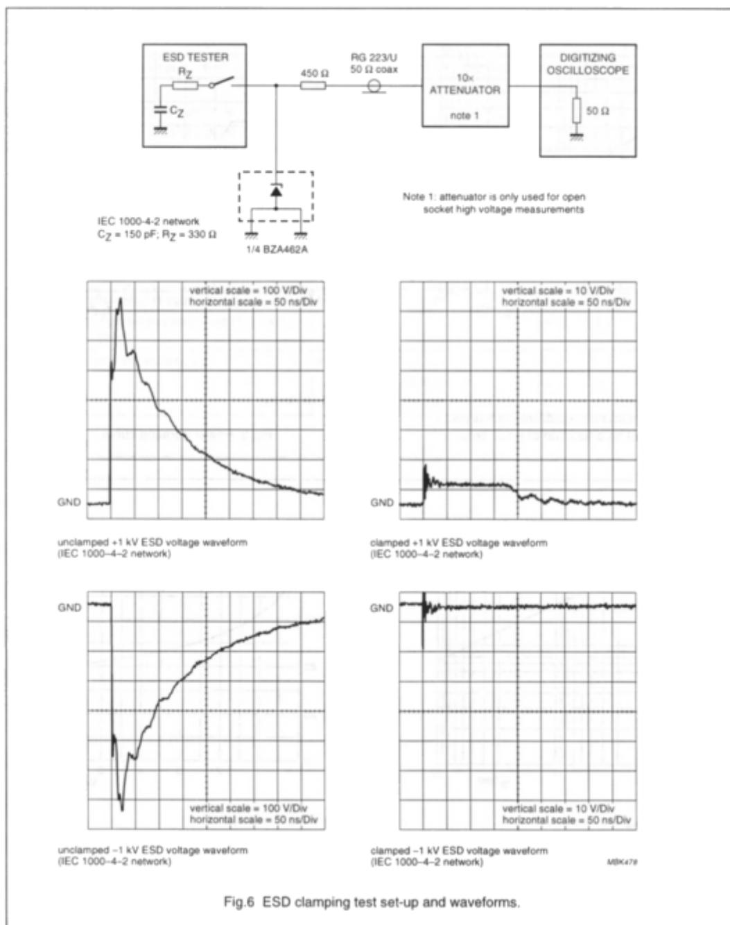
**Quadruple ESD transient voltage suppressor****BZA462A****APPLICATION INFORMATION****Typical common anode application**
