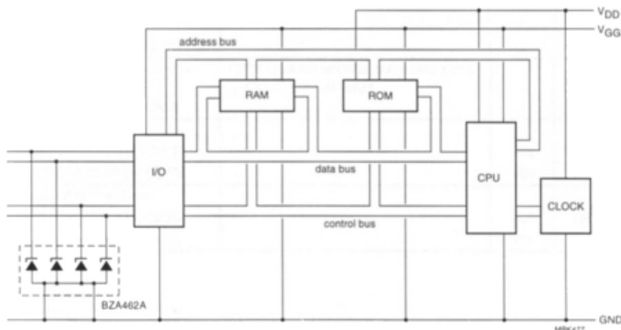
Fig.8 Microprocessor protection.
