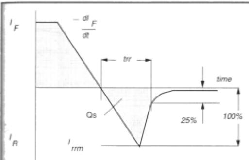
Fig.1. Definition of  $t_{rr}$ ,  $Q_s$  and  $I_{rrm}$
