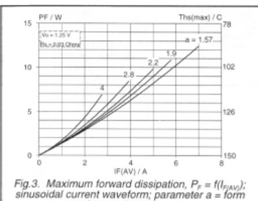
Fig.3. Maximum forward dissipation,  $P_F = f(IF_{(AV)})$ ;
