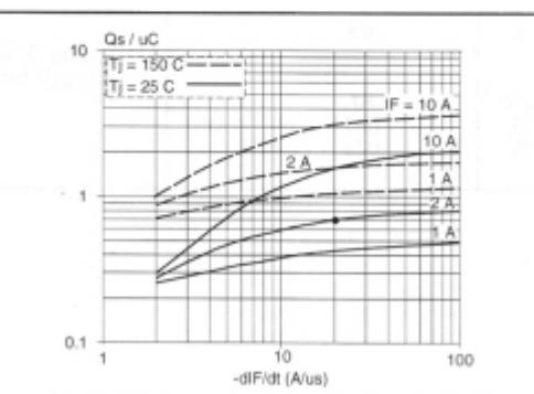
Fig.6. Maximum  $Q_s$  at  $T_j = 25^\circ\text{C}$  and  $150^\circ\text{C}$
