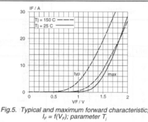
Fig.5. Typical and maximum forward characteristic;
