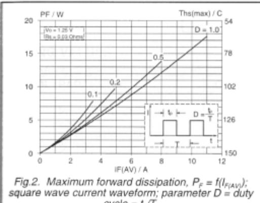
Fig.2. Maximum forward dissipation,  $P_F = f(IF_{(AV)})$ ;
