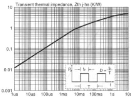
Fig.9. Transient thermal impedance  $Z_{th} = f(t_p)$
