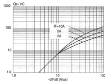
Fig.10. Maximum  $Q_s$  at  $T_j = 25^\circ C$ .
