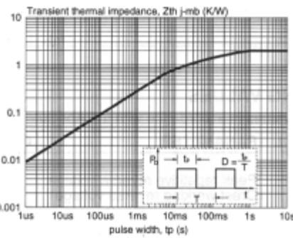
Fig.11. Transient thermal impedance;  $Z_{th\ j-mb} = f(t_p)$ .
