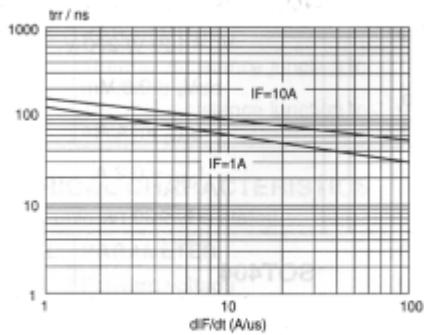
Fig.7. Maximum  $t_r$  at  $T_j = 25^\circ C$ .
