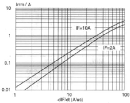
Fig.8. Maximum  $I_{rm}$  at  $T_j = 25^\circ C$ .
