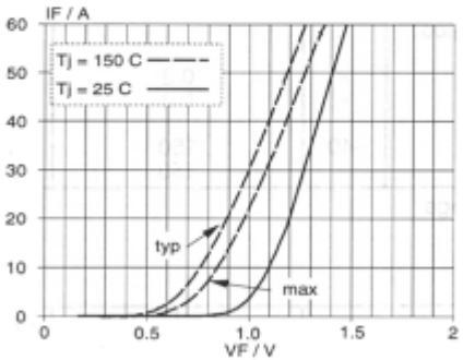
Fig.9. Typical and maximum forward characteristic
