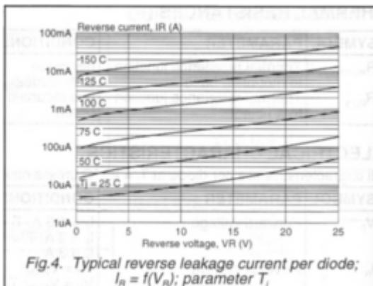
Fig.4. Typical reverse leakage current per diode;
