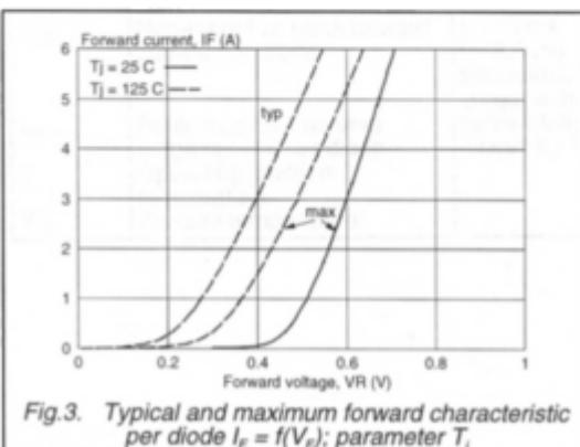
Fig.3. Typical and maximum forward characteristic per diode  $I_F = f(V_F)$ ; parameter  $T_j$
