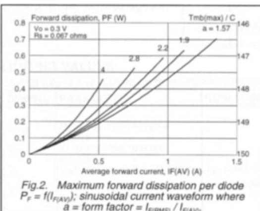
Fig.2. Maximum forward dissipation per diode
