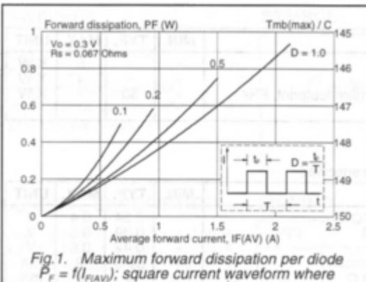
Fig.1. Maximum forward dissipation per diode
